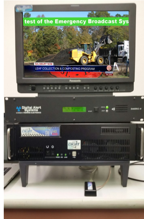
ChyTV HD EAS with Digital Alert Systems DASDEC II
